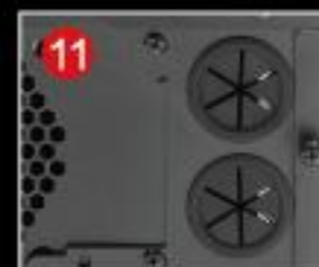
11 Pre-drill pipe holes for water cooling
