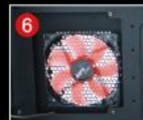
6 Can install 1x12cm fan on right side panel adjacent to CPU for added cooling per- formance
